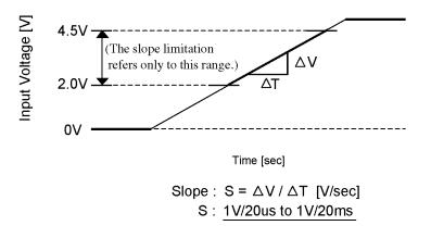
Figure 1.1 Permissible range of +5V rise slope
